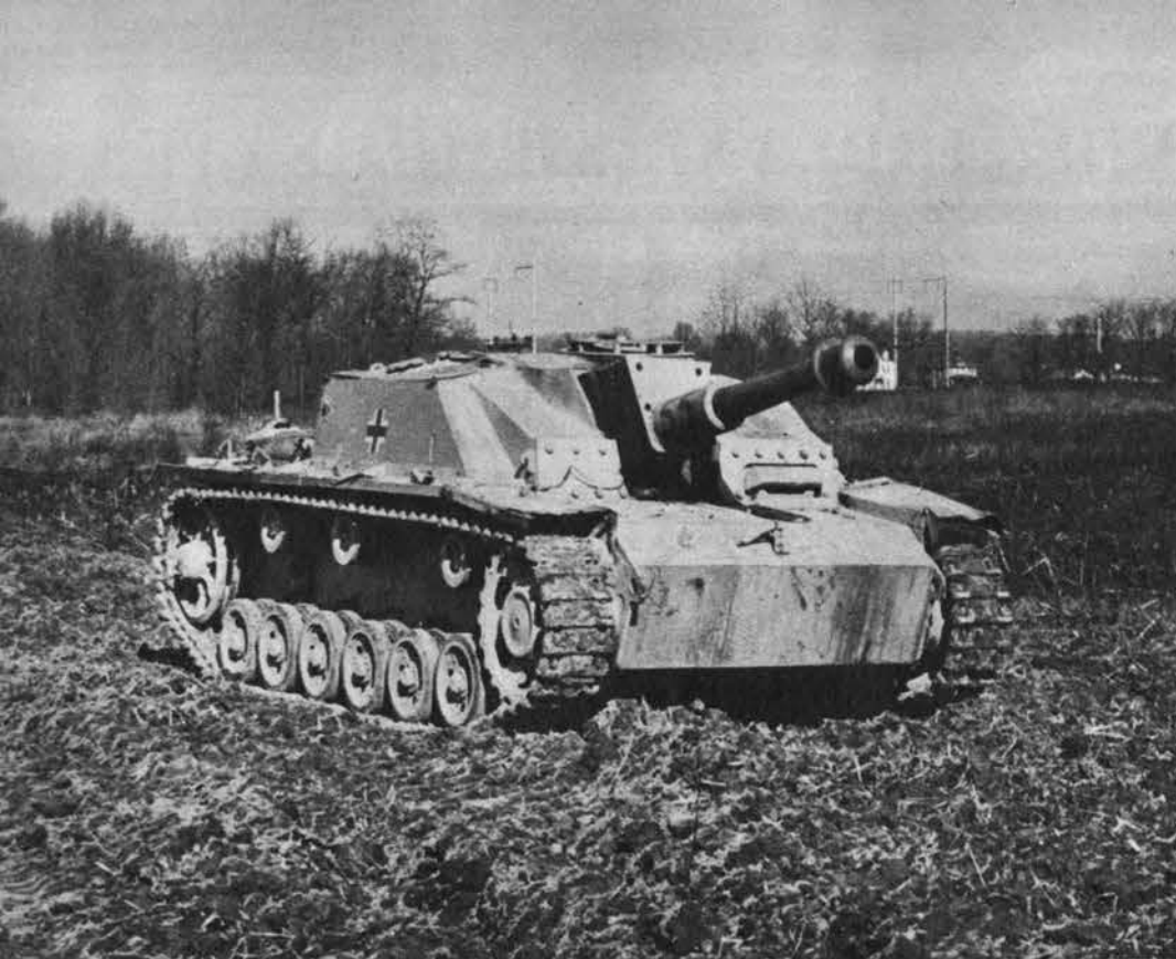
German medium assault gun is a thick-barreled 105-mm. gun mount on the chassis of the PzKw III tank. This weapon looks almost exactly like the 75-mm. Sturmgeschütz ( below ).
